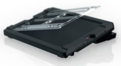
The keyguards are made from 5 mm thick plexiglass and can be supplied off-the-shelf or customized. They are milled instead of lasered to make sure the edges are **smooth and comfortable** for the user.
